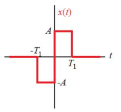
a. What is the total energy of the signal x(t) The total energy is given by:
